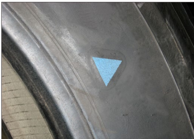
FIGURE 53: Blue Triangle Patch Applied to Sidewall
