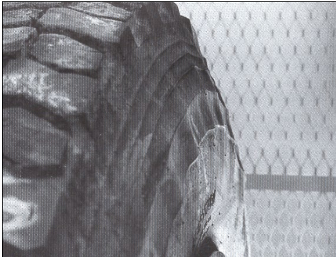
FIGURE 22: Using a grazing light or other indirect light source will produce shadows which indicate sidewall irregularities and/or signs of possible "zipper rupture."
