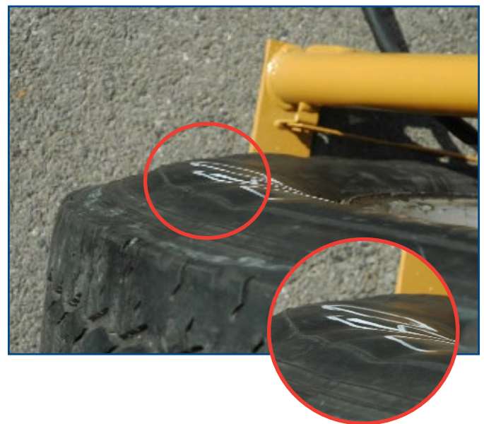
FIGURE 28: Undulating Rippled Sidewall 21
