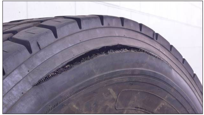
FIGURE 21: Example of a Zipper Rupture
